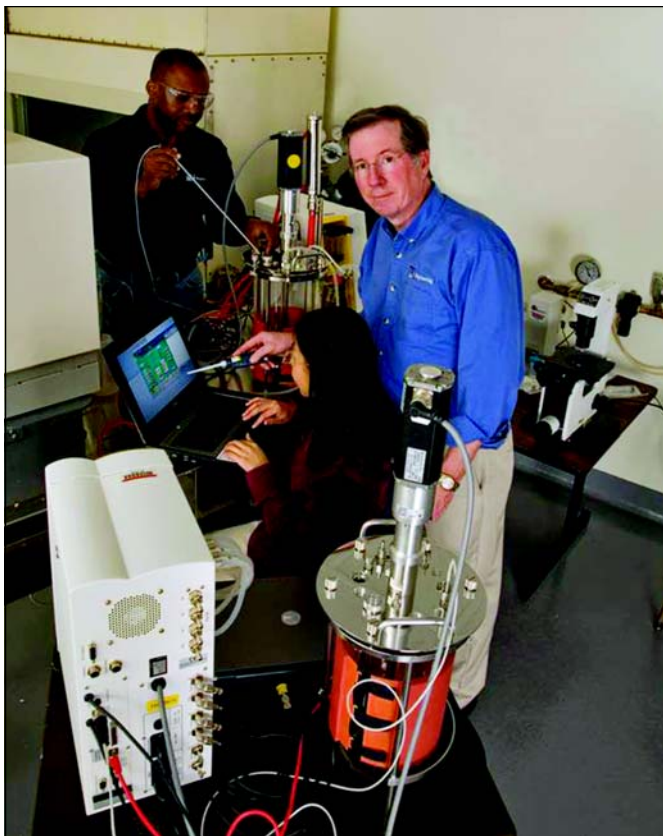
Dr. Carl Lawton, Director of Massachusetts BioManufacturing Center and staff analyze data for study of Glucose Feedback Control on CHO Cell Bioreactor.
