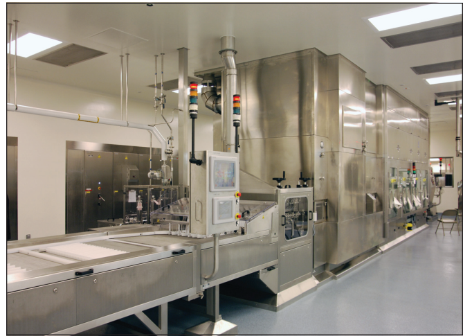
Figure 3. The fill line incorporated depyrogenation through capping within the isolator, including sterile stopper loading and automated lyo loading/unloading with all controls through an HMI.
