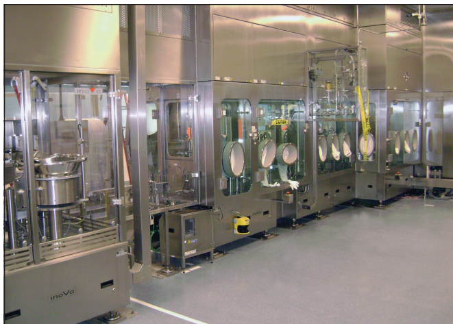
Figure 4. Isolator technology provides improved user comfort, due to reduced gowning requirements, while maintaining critical environmental control.
