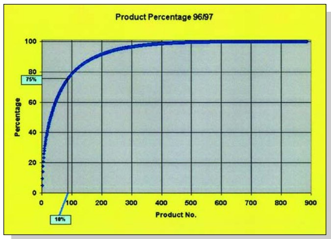
Figure 5. Cumulated packaging form percentages for one year. Nearly 900 different forms are packed.
