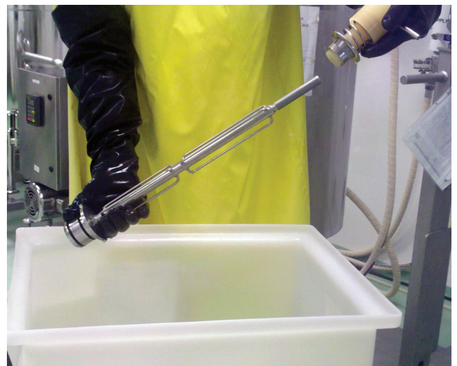
Figure 1. Manual washing utilizing soak tanks.
