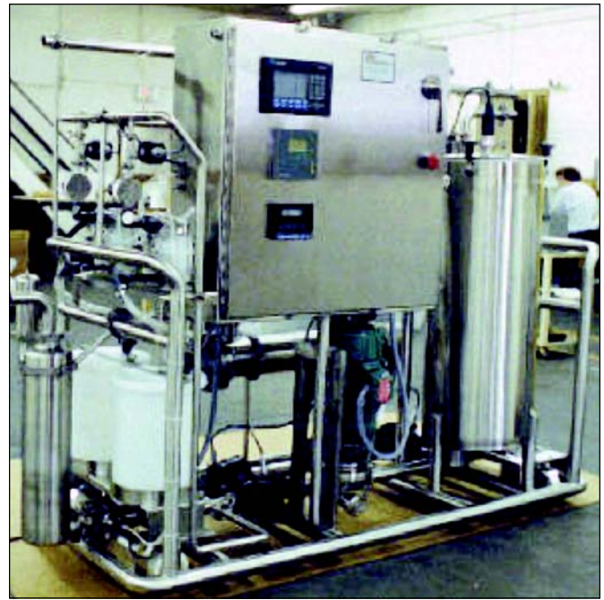
Figure 3. Portable CIP system. (Courtesy of Electrol Specialties Co.)
